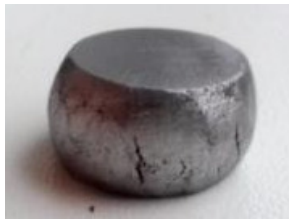
Fig. 4. Briquette after free sludge in the direction of initial pressing
