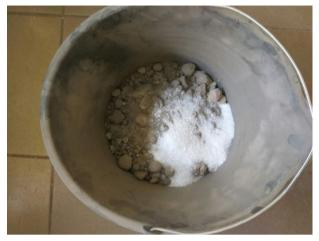
Fig. 2. Clinker and glass as a ball mill input
