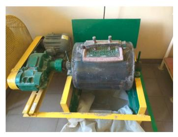
Fig. 1. Laboratory ball mill
