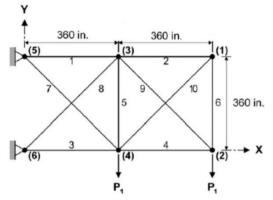
Fig. 2. Ten-bar planar truss
