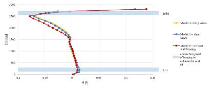
Fig. 7. The course of torsion angle variability along the column web length 63
