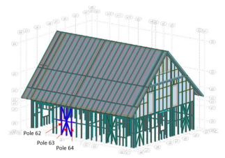
Fig. 2. Computational model of a single-family house construction in Autodesk Robot Structural 2015 with selected profiles for detailed analysis
