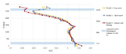
Fig. 8. The course of variability of the torsion angle along the length of the column shelf 63
