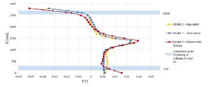
Fig. 10. The course of torsion angle variability along the length of the column shelf 64
