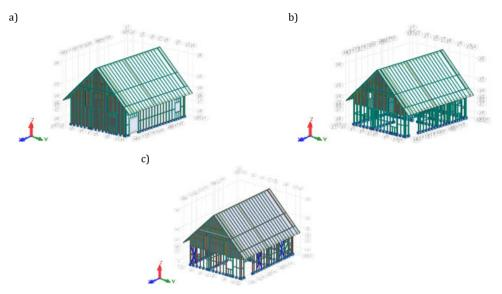
Fig. 1. Calculation models adopted: a) Model I - building structure with all sheathing, b) Model II
