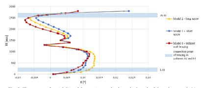
Fig. 9. The course of variability of the torsion angle along the length of the column web 64
