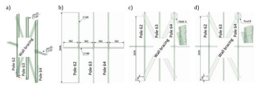
Fig. 3. Diagram of the wall section being analyzed: a) general view of selected profiles, b) Model 0 without bracing, c) Model 1 with bracing attached to one of the profile shelves (detail A), d) Model 2 with bracing attached by two profile shelves (detail B)
