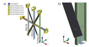
Fig. 4. Boundary conditions of the analyzed section: a) displacements applied at the center of gravity of the cross-section of the profiles, b) support in the form of anchoring the M10 anchor (example of a long bolt connection)
