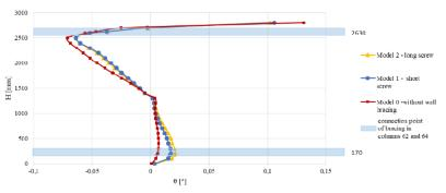
Fig. 5. The course of torsion angle variability along the column web length 62
