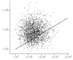
Fig. 7. Graphical representation of the integral (1) for the variant II of the analysis (vertical axis – maximum stress [Pa], horizontal axis – computed stress [Pa])
