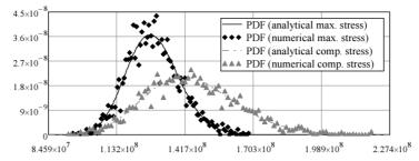
Fig. 6. Graphical representation of variant II of the analysis. The marginal probability density functions of the of calculated [Pa] and maximum [Pa] stresses (vertical axis – probability density [–], horizontal axis – stress [Pa])
