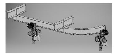
Fig. 3. An example solution of a curved on plane hoist beam suspended to the supporting structure
