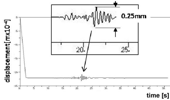
Fig. 10. Time dependent response of the vertical displacement in the "RBET" point of the shipping channel on sub-soil  $30 \text{ MNm}^{-3}$
