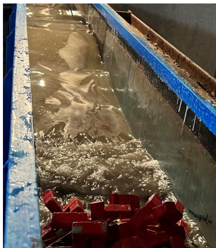
Fig. 2. "Gamma-Block" embankment test in the laboratory
